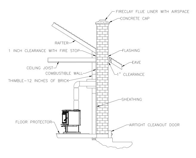
FIGURE 2.2.2 (A) Typical Installation Through an Existing Masonry Chimney
